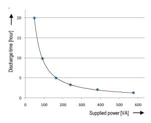
A monitor using 100Watt (100VA) can be provided with energy for about 10 hours.
